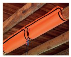
SAMITECH is revolutionising the pest control sector by improving classic heat treatments with a new technology based on far infrared waves that penetrate deep into the objects surface killing insects by dehydration.
