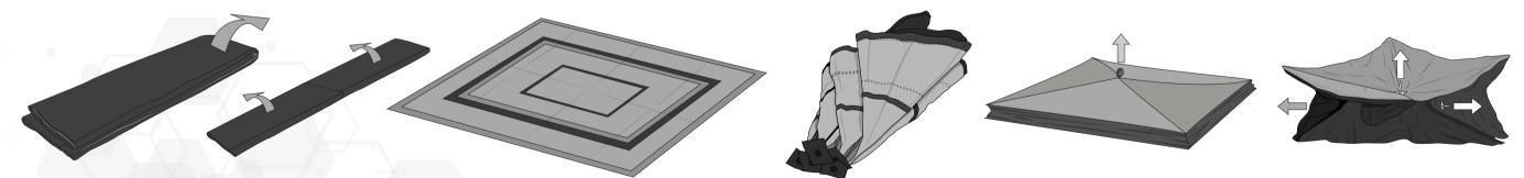
Open the Bubble by pulling the red strips. When the Bubble is standing and firm, place it over the base, sticking them with the Velcro tape. Finally, use the support poles to keep the Bubble open.
