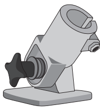
Tripod articulation unit
